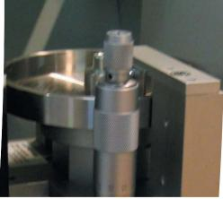
Stamping unit squeegee with selectable speed and adjustable epoxy film thickness
