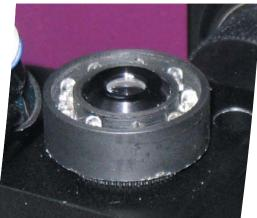
**Uplooking camera** with coaxial - and ring light for final accuracy optimization prior to placement
